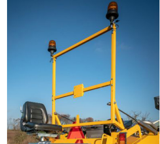
Bar with pneumatic lift for mounting warning lights (Comes without lights)
