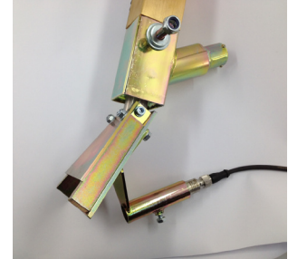
Bead alarm mounted on bead gun
