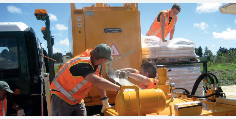
Borum thermoplastic preheaters are melting, heating and mixing the thermoplastic material making it ready for application via the road marking machine. They are provided either as a directly heated (D) or indirectly heated (ID).
