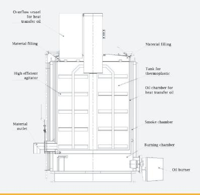
The preheaters are also equipped with a thermostat for thermoplastic material temperatures from +50 to +250 °C (+122 to 482 °F)
