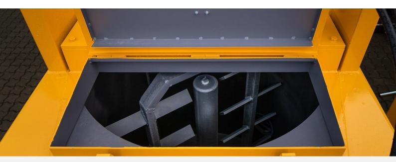
Both the direct and indirect preheaters are equipped with the high-speed agitator and mixing arms, which ensures a perfect mixing of the thermoplastic. The agitator is capable to turn both clock wise (CW) and counter-clockwise (CCW).
