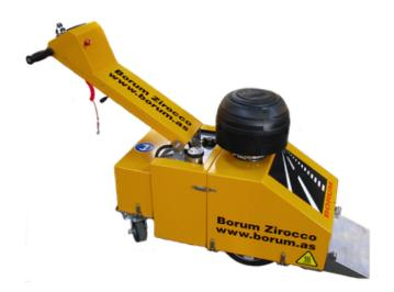
Many cities throughout the world have banned the use of open-flame and propane-powered road drying equipment. The Zirocco road dryer runs on a diesel fuelled 350 Kw microturbine. The micro-turbine has an output of 100 cubic metres of airflow per minute at up to 450-550 degrees Celsius. The machine is extremely effective for drying roads, removing black ice from tunnels and bridges, and removing chewing gum from public spaces.
