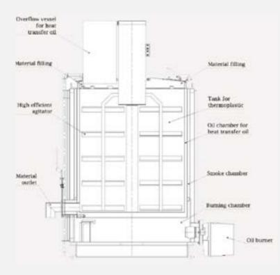
The preheaters are also equipped with a thermostat for thermoplastic material temperatures from +50 to +250  $^{\circ}$ C (+122 to 482  $^{\circ}$ F)
