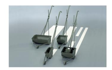
The Borum manual screed boxes can be used for marking one line up to 24 inch or a double line of 4 inch in one run. The thickness of the line can be from 0.06 to 0.2 inch . Antiskid material can be pre-mixed in order to make the markings less slippery.
