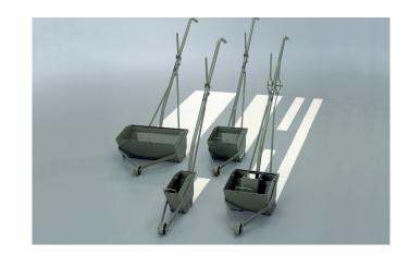
The Borum manual screed boxes can be used for marking one line up to 60 cm (24 inch) or a double line of 10 cm (4 inch) in one run. The thickness of the line can be from 1.5 mm to 5 mm (0.06 to 0.2 inch). Antiskid material can be pre-mixed in order to make the markings less slippery.
