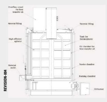
The preheaters are also equipped with a thermostat for thermoplastic material temperatures from +50 to +250  $^{\circ}$ C (+122 to 482  $^{\circ}$ F)
