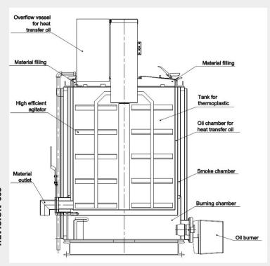
The preheaters are also equipped with a thermostat for thermoplastic material temperatures from +50 to +230°C
